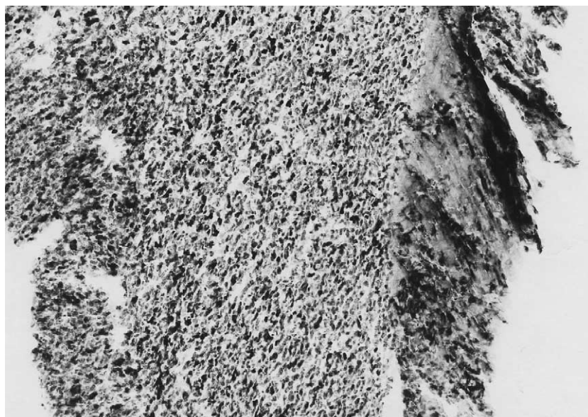
Fig. 2. TEM view of ultramicrotome cut of industrial Raney nickel aged after several recycling in glucose hydrogenation at 130 °C. The nickel micro-crystallites have sintered in the right-hand side of Raney nickel grain (unpublished results).
